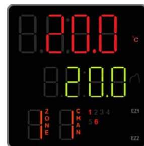
Figure 4: Unit operating in the manual night mode, as indicated by the "6"
