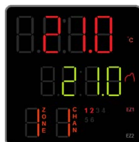
Figure 6: Operating in the auto cycle day phase, as indicated by the illuminated graph symbol and "2"
