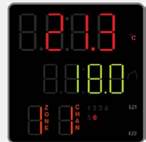
Manual night mode temperature set point adjusted. Cooling to the new set point.
