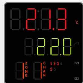
Day mode temperature set point adjusted. Heating to new set point
