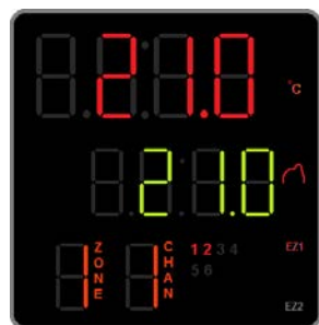
Figure 10: Home Page Cycle operating in the day phase The 2 indicates that the day illumination lights are active
