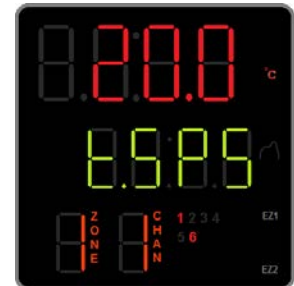
Initial Night Phase Temp. Set Point
